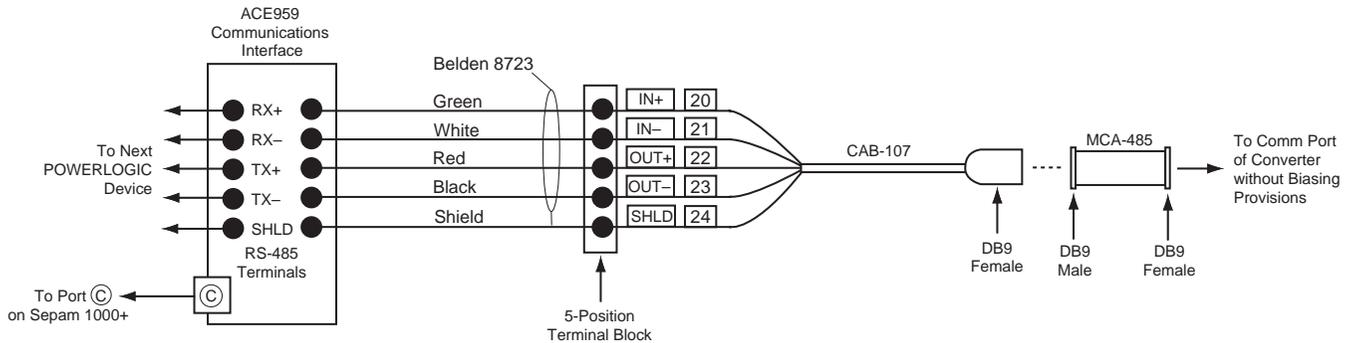
Connecting a Sepam 1000+ as the first device on a POWERLOGIC daisy chain using CAB107 cable, MCA-485, and terminal block
