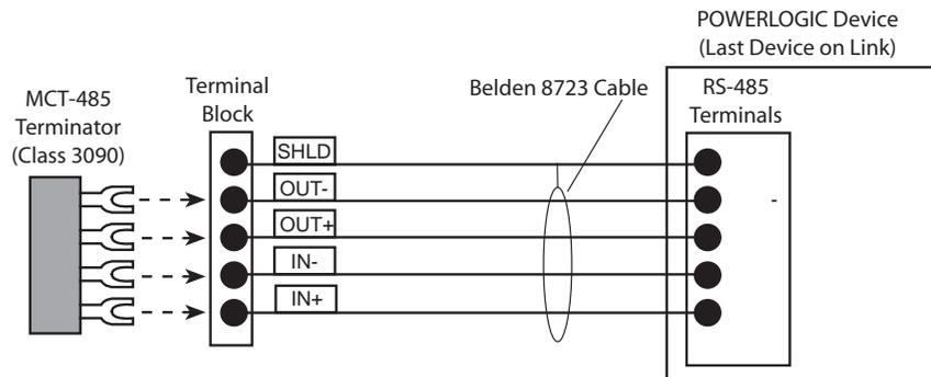
Terminating a device using an MCT-485 and a terminal block
