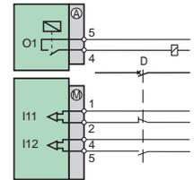
Wiring for undervoltage trip unit.
