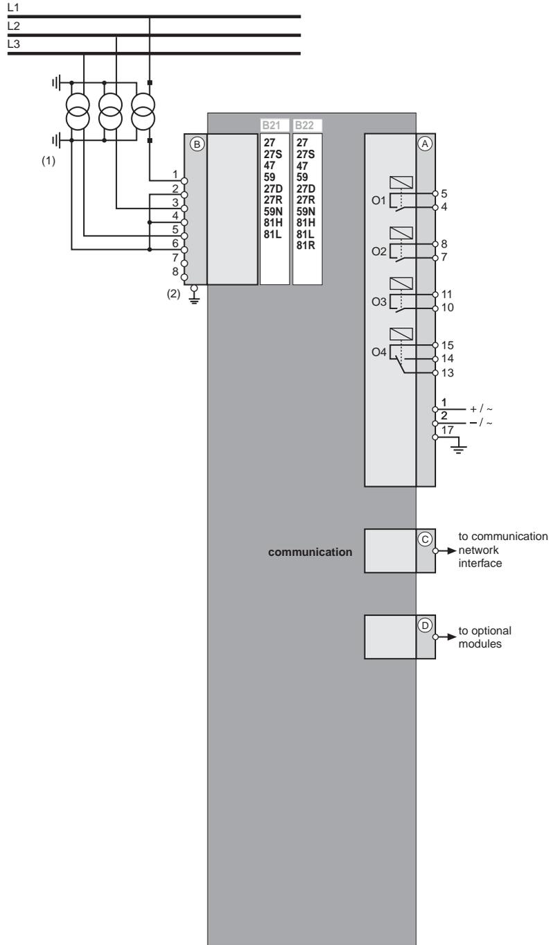
(1) This connection allows the residual voltage to be calculated.
