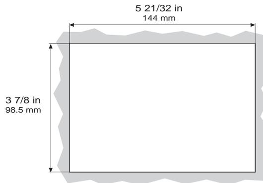
Cut-out dimensions for flush-mounting
