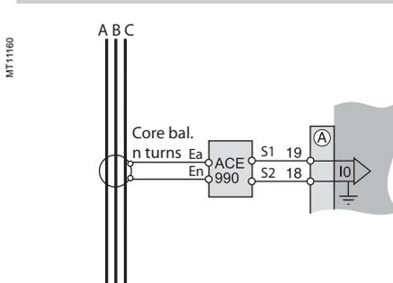
The ACE990 is used as an interface between a Medium Voltage core balance CT with ratio 1/n (50 < n < 1500) and the Sepam 1000+ residual current input. This arrangement makes it possible to keep the existing core balance CTs in the installation.
