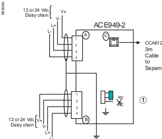
NOTE: When modules are linked together, the jumper ① should be put in the RC (load resistance) position on the last module in the series. The modules are delivered in the position ~~RC~~.
