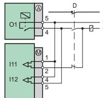
Wiring for shunt trip coil.
