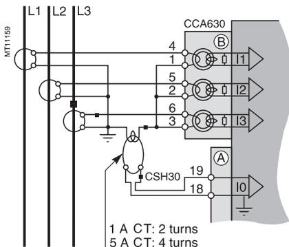
**Variant 4: residual current measurement by core balance CT with ratio 1/n (n between 50 and 1500)**
