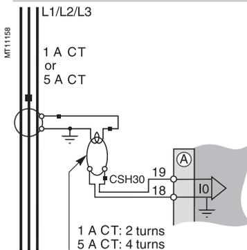
The CSH30 interposing ring CT is used to connect Sepam to 1 A or 5 A CTs to measure the residual current.
