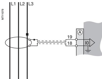
Arrangement recommended for the protection of isolated or compensated neutral systems in which very low fault currents need to be detected.
