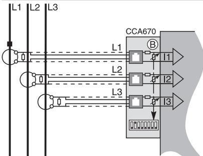
Connection of 3 Low Power Current Transducer (LPCT) type sensors to the CCA670 connector. The connection of just one or two sensors is not allowed.
