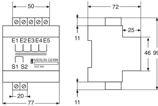
Mounted on symmetrical DIN rail, weight 640 g.
