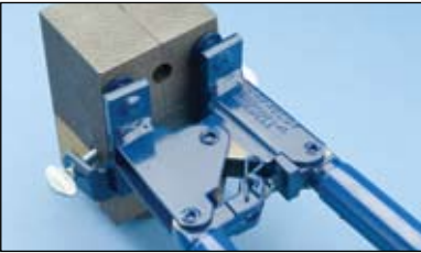
Fig. 8 Close the grips to tightly lock the mold. Check for an appropriate seal on the mold.
