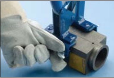
Fig. 7 Tighten the clamp thumbscrews onto the mold.
