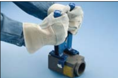
Fig. 9 If the mold does not seal properly, make adjustments to the handle clamp.
